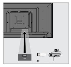
1 Connect the USB(HDD) USB interface on the television and the related data output on the external device (external hard disk, digital camera, card reader or MP3 player) with a USB cable;
